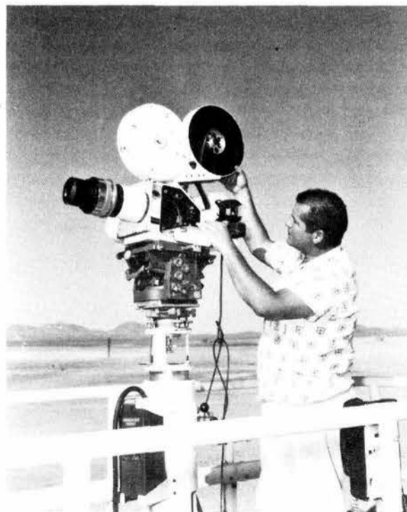
THREADING A 35-mm Photosonics (high-speed motion picture camera) is Joe Durrenberger (ret.); he was one of several photo-technicians at TTR in the 60s.
